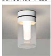
**Technical:** 12W LED | 1200Lm (Light source) 600Lm (luminaire) | CRI 80 | 3000K | Included Control Gear | 100-240V | IP54
