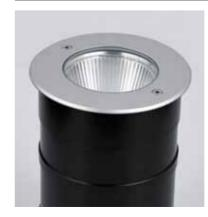
Technical: 22W LED CREE | 1665Lm (light source) 1451Lm (Luminiare) | CRI 85 | 15°, 24°, 36° | 3000K-6000K | HEP Control Gear | 100-277V | IP67
