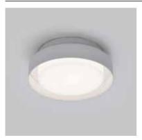
**Technical:** 15W LED | 1000Lm (light source) 620 (Luminaire) | CRI 80 | 3000K -6000k | Included Control Gear | 220-240V | IP54
