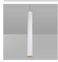
**Technical:** 5W LED Bridgelux | 440Lm (light source) 315Lm (luminaire) | CRI 80 | 24°, 36° | 3000K | HEP Control Gear | 220-240V | IP20
