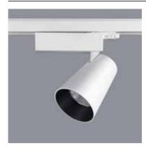
**Technical:** 24W LED Lumileds | 3000Lm (light source) 2250Lm (luminaire) | CRI 90 | 17°, 25°, 35°, 50° | 2700K, 3000K, 4000K | Osram Control Gear | 220-240V | IP20
