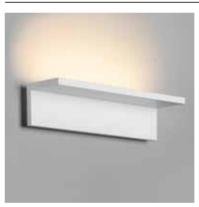
**Technical:** 11W LED OSRAM | 1485Lm (light source) 1100Lm (luminaire) | CRI 80 | 3000K, 4000K | Tridonic Triac Dimmable Control Gear | 220-240V | IP20
