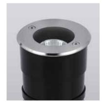
**Technical:** 8W LED CREE | 687Lm (light source) 533Lm (Luminiare) | CRI 85 | 15°, 24°, 36° | 3000K-6000K | HEP Control Gear | 100-240V | IP67
