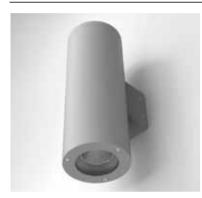
**Technical:** 31W LED Cree | 2493Lm (light source) 2200 (Luminaire) | CRI 85 | 15°, 38°, 60° | 3000K-6000K | HEP Control Gear | 220-240V | IP65
