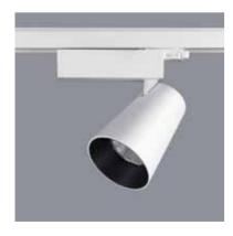
**Technical:** 37W LED Lumileds | 4625Lm (light source) 3490Lm (luminaire) | CRI 90 | 17°, 25°, 35°, 50° | 2700K, 3000K, 4000K | Osram Control Gear | 220-240V | IP20
