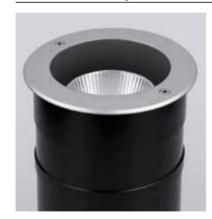
**Technical:** 22W LED CREE | 1555Lm (light source) 1010Lm (Luminiare) | CRI 85 | 15°, 24°, 36° | 3000K-6000K | HEP Control Gear | 100-277V | IP67
