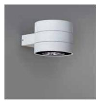
**Technical:** 14W LED CREE | 1470Lm (Light source) 1260Lm (Luminaire) | CRI 80 | 12°, 24°, 36° | 3000K, 4000K | Included Control Gear | 100- 240V | IP65
