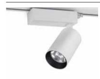
**Technical:** 24W LED Lumileds | 3000Lm (light source) 2510Lm (luminaire) | CRI 90 | 25°, 35°, 45° | 2700K, 3000K, 4000K | Osram Control Gear | 220-240V | IP20
