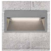
**Technical:** 10W LED | 600Lm (Light source) 400Lm (Luminaire) | CRI 80 | 3000K-6000K | Tridonic Control Gear | 220-240V | IP54
