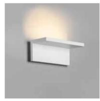
**Technical:** 13W LED OSRAM | 1755Lm (light source) 1350Lm (luminaire) | CRI 80 | 3000K, 4000K | Tridonic Triac Dimmable Control Gear | 220-240V | IP20
