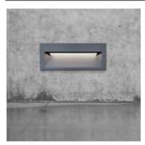
**Technical:** 4W LED | 240Lm (Light source) 120Lm (Luminaire) | CRI 80 | 3000K-6000K | Included Control Gear | 220-240V | IP65
