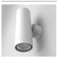
**Technical:** 11W LED CREE | 1023Lm (light source) 840Lm (Luminiare) | 15°, 25°, 35° | 3000K-6000K | HEP Control Gear | 100-240V | IP65
