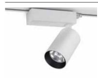
**Technical:** 37W LED Lumileds | 4625Lm (light source) 3890Lm (luminaire) | CRI 90 | 25°, 35°, 45° | 2700K, 3000K, 4000K | Osram Control Gear | 220-240V | IP20
